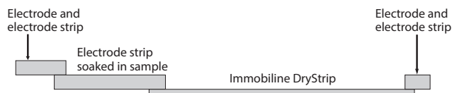
Fig 1. Preparative sample application using paper-bridge loading
