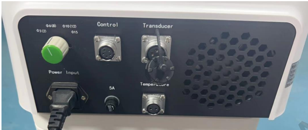
Rear panel of the generator showing cable locations
