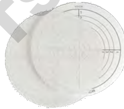
Picture 4: transparent and white diffusing counting grids
