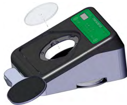
Picture 7: Removing the glass
