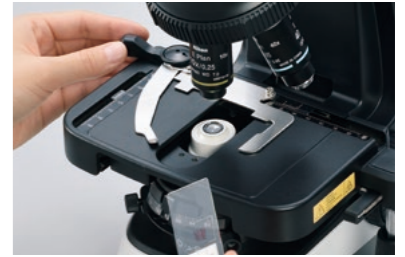
Easy-to-operate specimen holder
