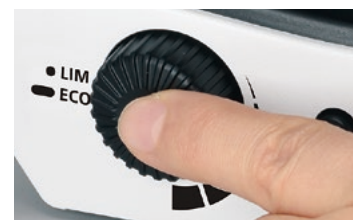
Push the brightness control knob briefly to activate the LIM feature.
