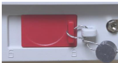
Locked with Wire Seal
