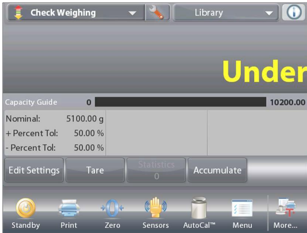
The CHECK WEIGHING home screen with Display set to Check Status
