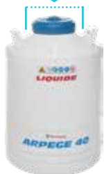
ARPEGE model with narrow neck for a longer holding time
