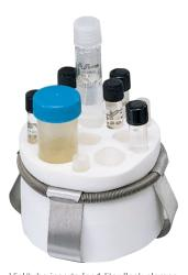
Vial/tube inserts for 1 liter flask clamps
