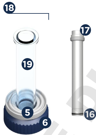
Figure 4 Aspiration system, located under outer housing
