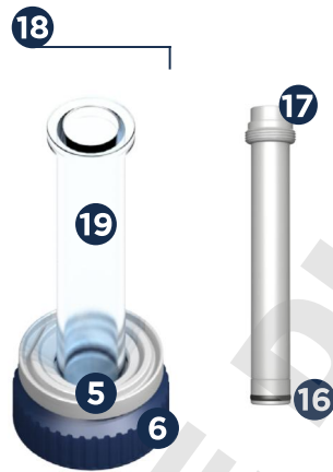
Figure 4 Aspiration system, located under outer housing
