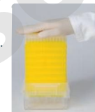
Place the tower on the reload box and press down firmly with your hand.
