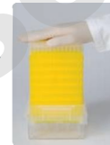
Place the tower on the reload box and press down firmly with your hand.
