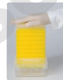
Place the tower on the reload box and press down firmly with your hand.
