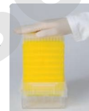
Place the tower on the reload box and press down firmly with your hand.
