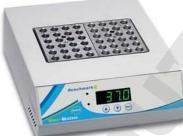
The Benchmark series of digital dry baths offer digital control over both temperature and time, eliminating the need for an external thermometer or timer. Available in three configurations, the digital dry baths offer capacity for up to four blocks. They are extremely space efficient. (The four block model can accommodate up to 96x1.5ml tubes in less than a square foot of bench space.)
