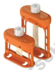
Micro Float-A-Lyzer® ready-to-use dialysis devices are all made with proprietary Biotech Grade CE dialysis tubing, preassembled with volume specific lengths of membrane tubing and designed to maximize convenience, ease-of-use and sample recovery.
