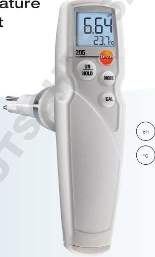
The testo 205 is a robust food penetration measuring instrument for temperature and pH values, with automatic temperature compensation. The robust penetration measurement tip is exchangeable and insenstitive to dirt thanks to the hole diaphragm.
