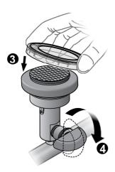
4. Remove the base from the filtration head as shown here:
