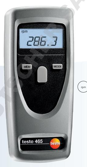
With the testo 465, you can measure rpm easily without contact using only one hand. The measuring instrument is thus suitable for measurements on rotating parts such as ventilators and shafts. Simply attach a reflective marker (optional) to the measurement object, point the visible red beam of light at the reflective marker, and measure. The
