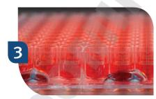
Evaporation takes place in the moat and not the outer wells - preserving cell viability and maintaining well-to-well consistency
