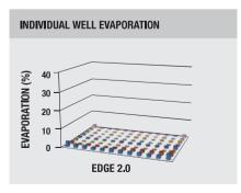
The built-in moat in the Nunc Edge 2.0 Plate effectively eliminates edge effect in the perimeter wells caused by evaporation.
