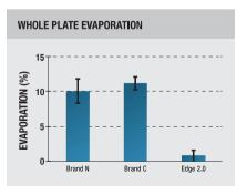
The built-in moat in the Nunc Edge 2.0 Plate significantly reduces whole plate evaporation as compared to conventional 96-well plates
