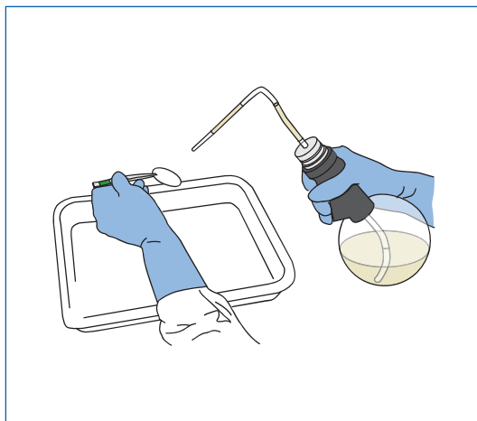
Figure 26. Flushing filter with solvent filtering dispenser.
