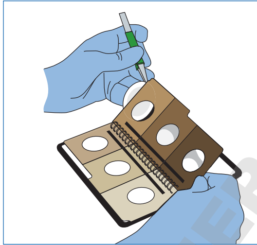
Figure 53. Comparing patch obtained on filter removed from fluid sampling cassette to standard colored patches (of known contaminant levels) contained in patch test booklet.
