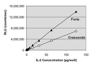
Substrate sensitivity was determined using IL-2 sandwich ELISA. Recombinant mouse IL-2 was serially diluted in a white 96-well plate and detected using IL-2 ELISPOT antibody pair (Millipore cat. no. ELI-002-M). Luminescence was measured using a Wallac VICTOR<sup>2™</sup> 1420 multilabel counter.
