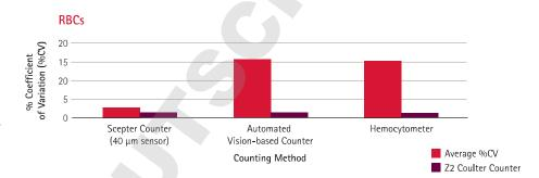
The Scepter 2.0 cell counter counts RBCs with greater precision than other counting methods, as reflected by low coefficients of variation. %CVs were calculated using average cell counts of four replicate samples.
