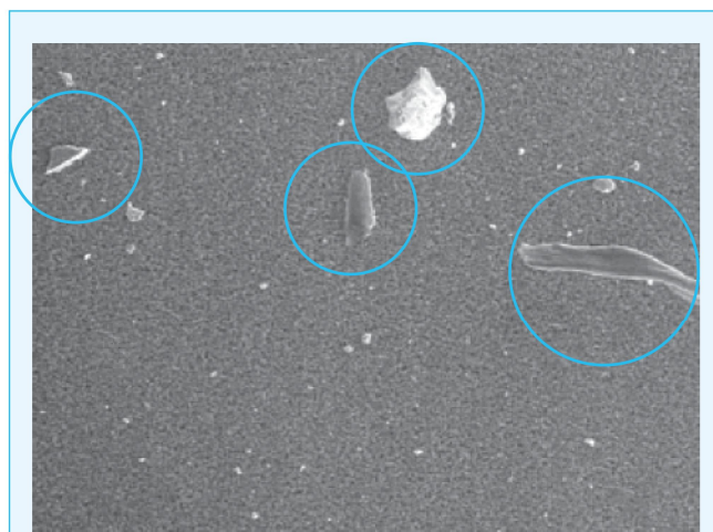
Figure 1. Particles trapped on a 0.2 \mu\text{m} PVDF membrane filter after filtration of 2 L of 50 mM sodium bicarbonate buffer. If the buffer were not filtered before running through the column, these particles could contaminate and clog the expensive UHPLC column.
