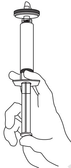
Hold the syringe with filter pointing up and “top off” by pushing a few drops through the filter.
