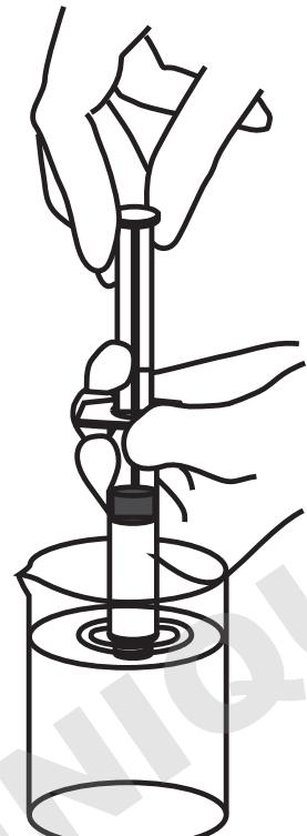
Fill the syringe with the solution to be filtered.
