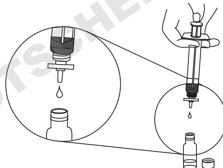
Push the syringe plunger to deliver a filtered solution.
