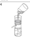
Remove lid (if not already removed) and pour sample into funnel. Replace lid, if desired, and apply vacuum until filtration is complete.
