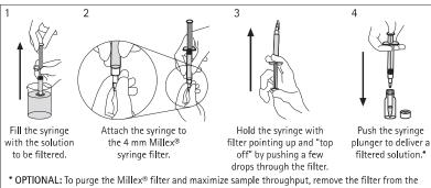
\* OPTIONAL: To purge the Millex® filter and maximize sample throughput, remove the filter from the syringe and draw air into the syringe. Then reattach the filter and push the plunger to force some of the air through the filter.
