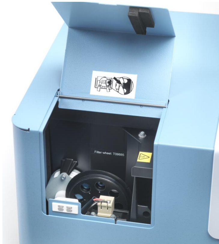
Figure 19. Removing the filter wheel
