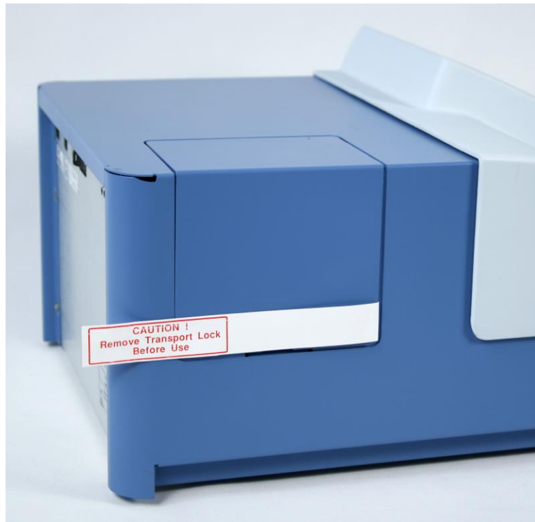
Figure 29. Transport lock bar and tag refitted
