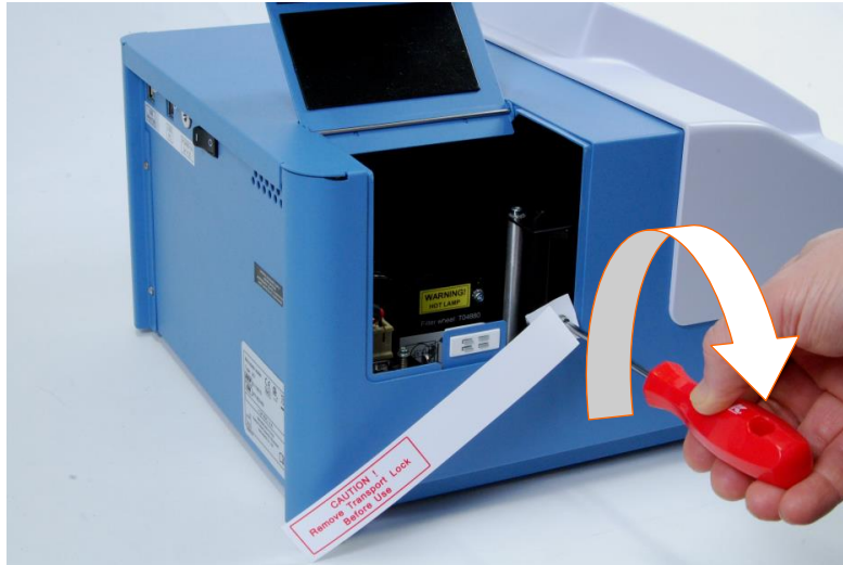
Figure 28. Fastening the transport lock
