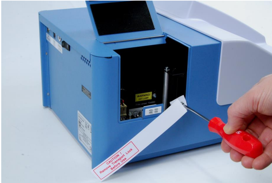
Figure 4. Unfastening the transport lock
