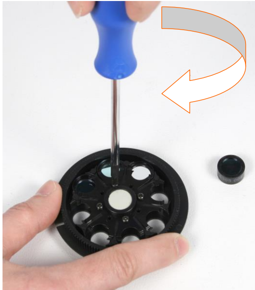
Figure 20. Removing the spring position holding screws
