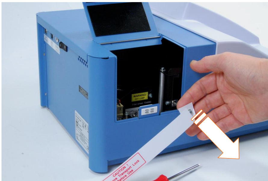
Figure 5. Pulling the transport lock out
