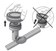
5. Replace the plug and twist it onto the support.
