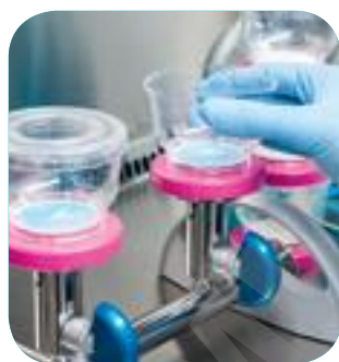
EZ-Fit® Filtration Unit set-up
