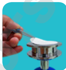
Placing filter on manifold head
