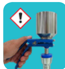
Installing filter funnel on manifold
