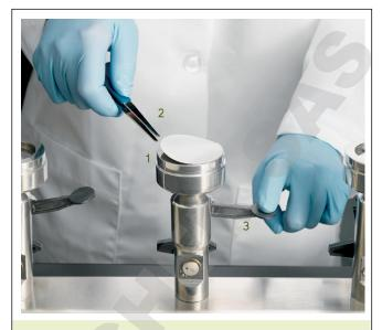
The unique sealing lip of the Microfil funnel avoids the risk of membrane by-pass by microorganisms. The clipping (1) holds the funnel firmly on the filtration support. After filtration, the funnel is removed and the membrane is lifted together with the membrane support (2) by simply pressing the lever (3). The membrane can now be conveniently removed from the support using forceps.
