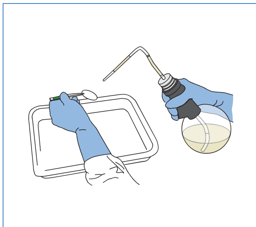
Figure 26. Flushing filter with solvent filtering dispenser.
