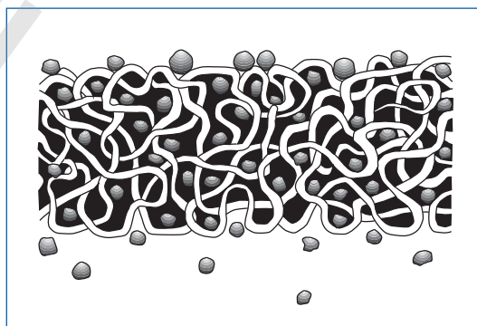
Figure 2. Schematic cross section, depth filter. Random entrapment of particles.
