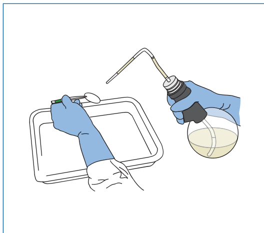
Figure 26. Flushing filter with solvent filtering dispenser.
