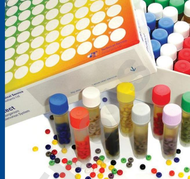
**Protect** - the original low temperature bead storage system, ideal for long term maintenance of stock and quality control microorganisms. Each vial provides 20 subcultures, dramatically reducing the cost per test versus other techniques.
