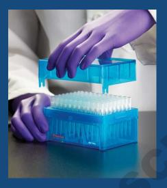
Turn the cover so the hinges align to front of the rack.
