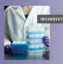
Plastic sleeve is not intended to rest on any counter top without a rack underneath it.
