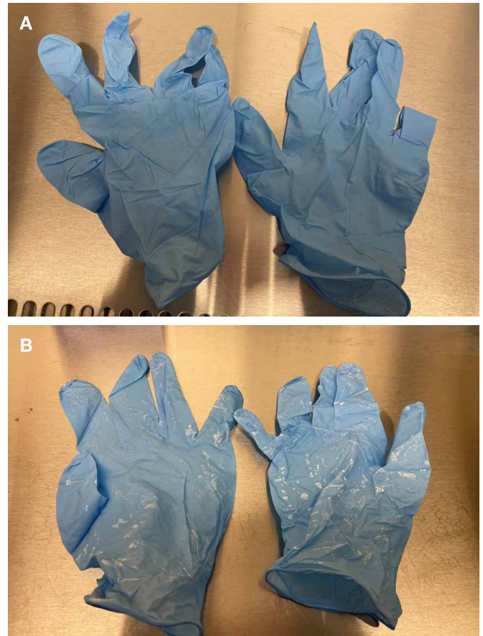
Figure 3. Laboratory gloves dried after decontamination. Gloves were sprayed with (A) RNase AWAY reagent and (B) bleach.
