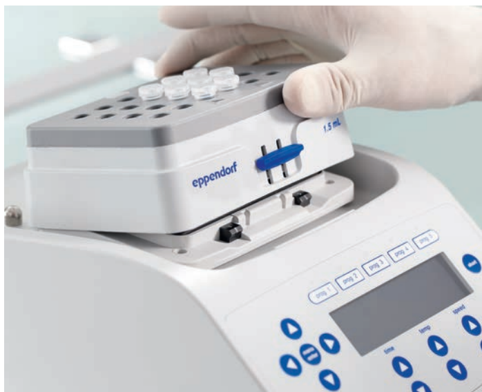
SmartBlock removal from Eppendorf ThermoMixer® C
