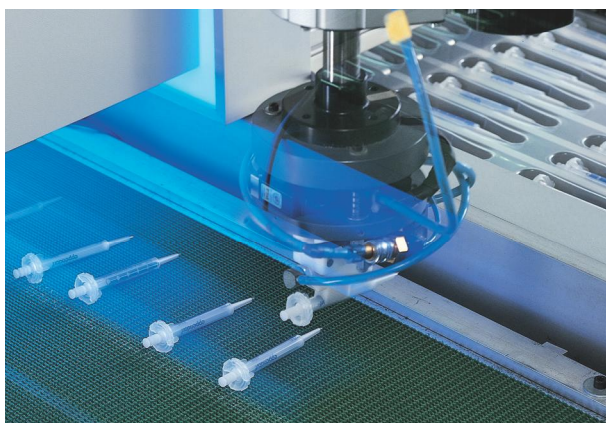
Fig. 2: Fully automatic sorting of Combitips into blister packs under clean-room conditions.
