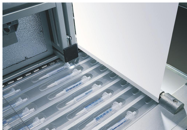
Fig. 3: Packing of consumables with Eppendorf purity grade Eppendorf Biopur prior to sterilization
