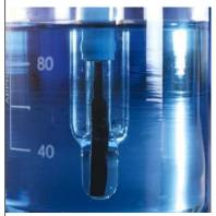
Upon connection of any InLab ISM (Intelligent Sensor Management) sensor, the instrument automaticaly recognizes the sensor and stores sensor ID, serial number, and last calibration data. This reduces the time needed to setup the instrument and reduces chances of error thanks to correct sensor identification.
