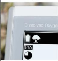
The outdoor user mode, which comes in addition to the routine and expert laboratory modes, provides users with default instrument settings (e.g. screen brightness sleep mode, and auto-shutdown) that ensure the Seven2Go portable's battery lasts, even if the nearest AA batteries are miles away.
