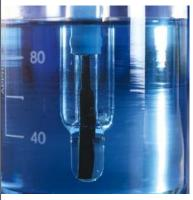
Upon connection of any InLab ISM (Intelligent Sensor Management) sensor, the instrument automaticaly recognizes the sensor and stores sensor ID, serial number, and last calibration data. This reduces the time needed to setup the instrument and reduces chances of error thanks to correct sensor identification.
