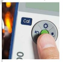
Seven2Go's new T-pad hardkey buttons with clicker technology improve the speed with which you move through menus and set measurement parameters. The intuitive and faster navigation shortens the time to actual measurement.
