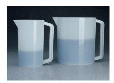
Nalgene™ HDPE Beakers with handles feature an extra-heavy wall for safe handling of acids, alkalis and hot solutions.
