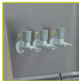
Media taps mounted on rear wall
