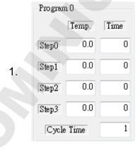
There are 4 setting steps, from step 0 to step 3 for temperature (Temp.) and operation time (Time) setting, and also setting for Cycle Times.
