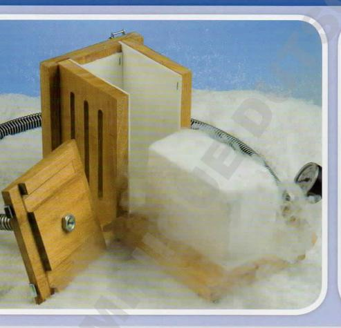
The 'DILVAC' Portable Dry-ice maker works on the principle of Adiabatic expansion (the Joule-Thompson effect). The liquid CO<sub>2</sub> in the cylinder is at a pressure greater than 60 Kg/cm2, so when it is released into the unit, which is at atmospheric pressure, the liquid CO<sub>2</sub> vaporises and expands. As a result of this expansion, the liquid changes to snow and is compacted into a block within the unit. The block measures 80mm x 110mm x 180mm and weighs approx. 1 Kg.
