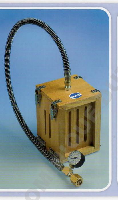
The 'DILVAC' Portable Dry-Ice maker is the fastest way of providing a block of Dry-Ice to your lab. It is compact and lightweight, requires no electric power and is safe and simple to use. Most importantly, it is always there in the lab to give you immediate access to Dry-Ice WHEN YOU NEED IT. The economy of having your Dry-lce 'on tap' can provide considerable financial savings over a relatively short period as the cost of having Dry-Ice delivered to your lab can be prohibitive.
