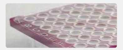
The PCR seal is a durable transparent polyester film with a strong adhesive layer. This seal enables a high seal integrity and efficiently prevents sample evaporation. It is recommended for PCR, qPCR and other optical applications (e.g. fluorescence or colorimetric measurements) as well as sample storage.
