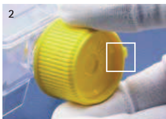
1 Aeration position of «VENT» screw cap, 12 o'clock.
