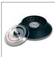
18 x 1.5 mL fixed angle rotor (Cat. No. 480139)
